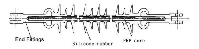
Fig. 33KV 70KN Composite Deadend Insulator
